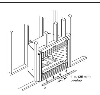
Protective metal strips are placed 2 in. (51 mm) under the front of the fireplace and must extend beyond the front and sides of fireplace opening by 2 in. (51 mm).
